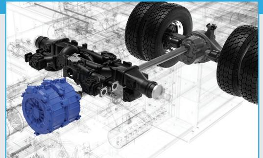
**FULLY ELECTRIC DRIVE AND PUMP OPERATIONS—OVER TWO HOURS PUMPING AT 1250 GPM (4730 LPM) FROM DRAFT**
